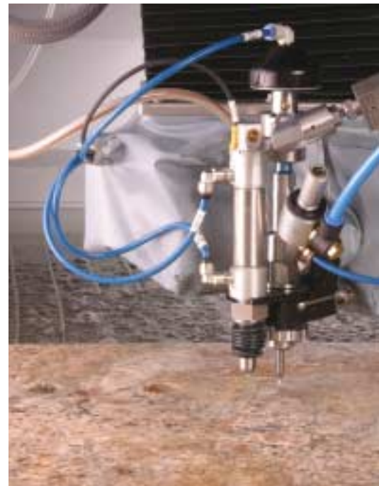
Flow waterjets are used for difficult and complex cuts.
